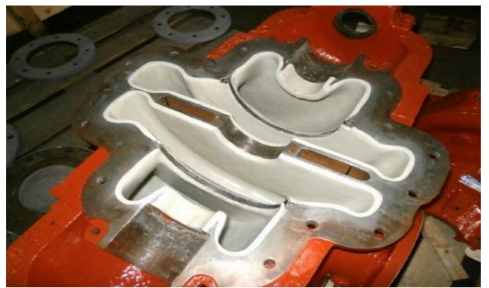
Refurbishment of horizontal split casing fire pump and protective lining with Corroglass 600 coating.
