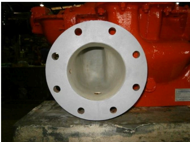
Refurbishment of horizontal split casing fire pump and protective lining with Corroglass 600 coating.
