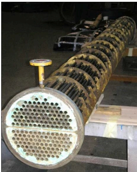
Example of a tube bundle cleaned and refurbished along with water box.
