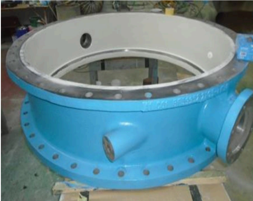
An example of a newly fabricated Butterfly valves corrosion protected.
